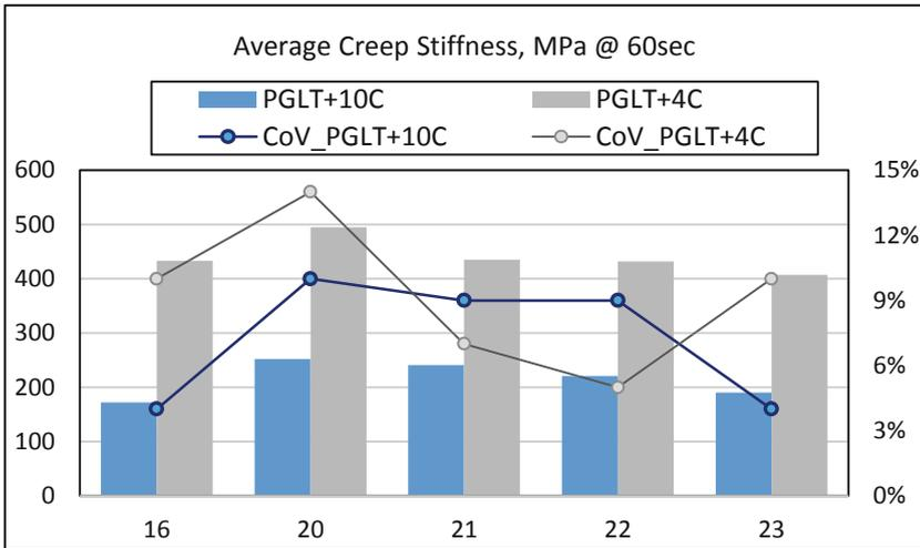
Fig. 5. BBR creep stiffness at 60 s for binders from Cell 16, 20–23.
