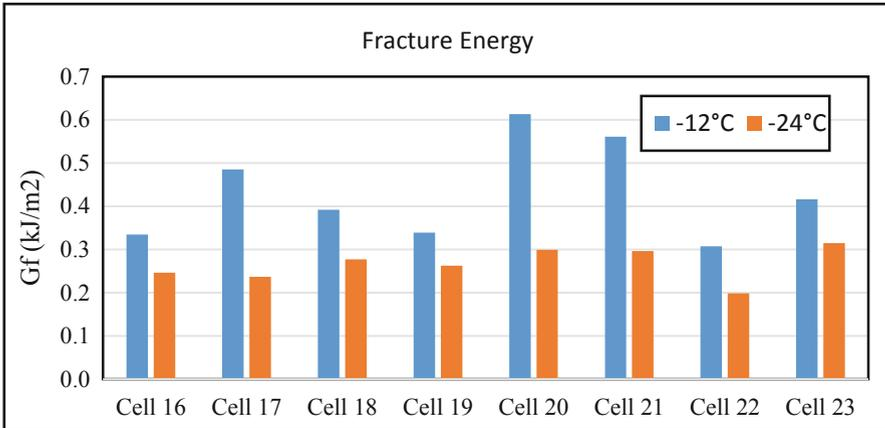
**Fig. 3.** SCB fracture energy for all mixtures.
