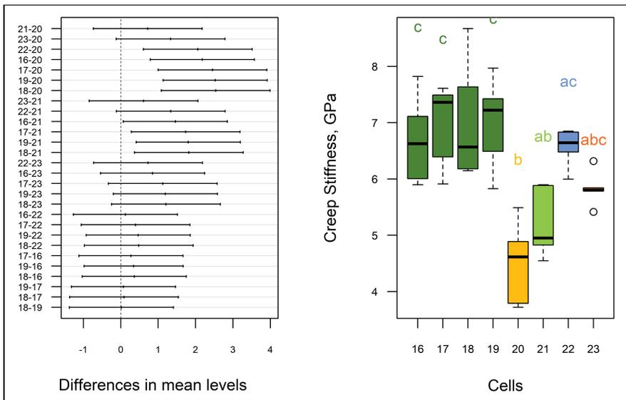
Fig. 7. (a) Confidence intervals (Tukey) for BBR creep stiffness at  $-12\text{ }^{\circ}\text{C}$ .
