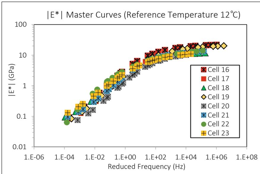
**Fig. 4.** IDT  $|E^*|$  master curves of all mixtures.
