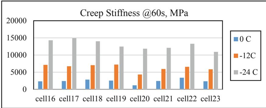
Fig. 1. BBR creep stiffness at 60 s of all mixtures.
