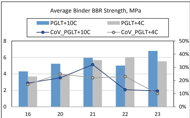
Fig. 6. BBR strength for binders from Cell 16, 20–23.
