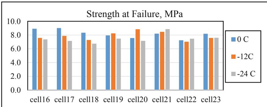
Fig. 2. BBR strength of all mixtures.
