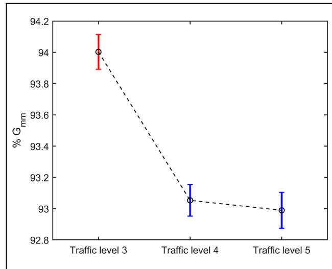
**Figure 8.** Comparison between mixtures grouped by different traffic levels. Note:  $G_{mm}$  = theoretical maximum specific gravity.
