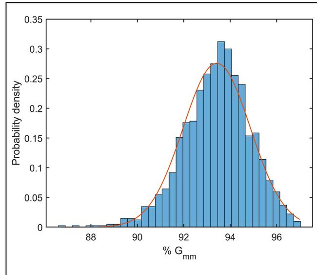
**Figure 3.** Probability distribution of field density data. Note:  $G_{mm}$  = theoretical maximum specific gravity. The red curve is a normal distribution regression of the data.
