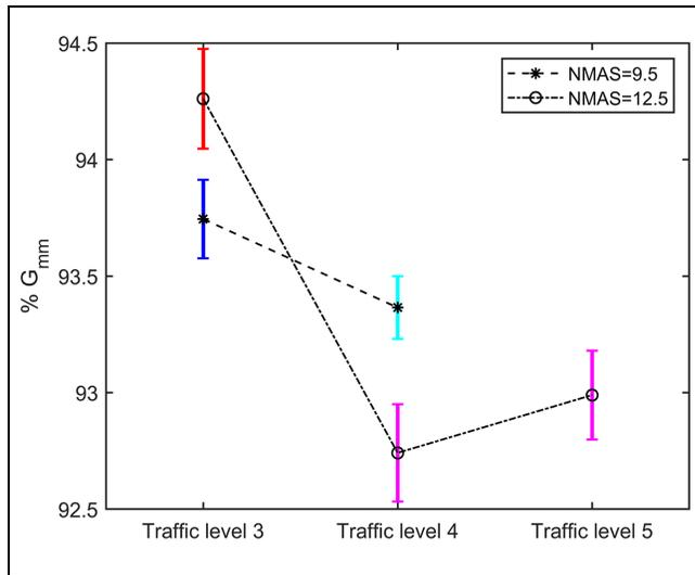
**Figure 9.** Comparison between mixtures grouped by both nominal maximum aggregate size (NMAS) and traffic level. Note:  $G_{mm}$  = theoretical maximum specific gravity.
