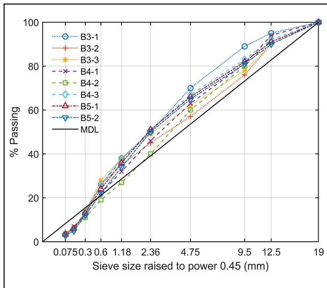
**Figure 2.** Gradation curves of mixtures with nominal maximum aggregate size (NMAS) = 12.5 mm.
