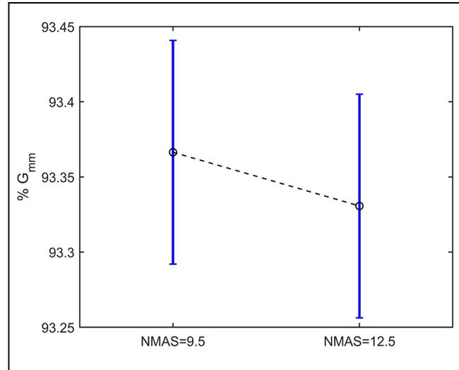
**Figure 7.** Comparison between mixtures grouped by different nominal maximum aggregate size (NMA) levels. Note:  $G_{mm}$  = theoretical maximum specific gravity.
