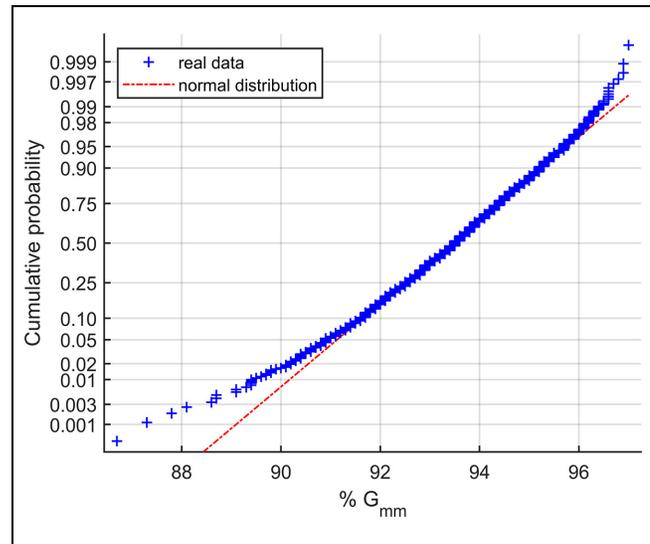
**Figure 4.** Normal distribution quantile-quantile plot for field density data. Note:  $G_{mm}$  = theoretical maximum specific gravity.
