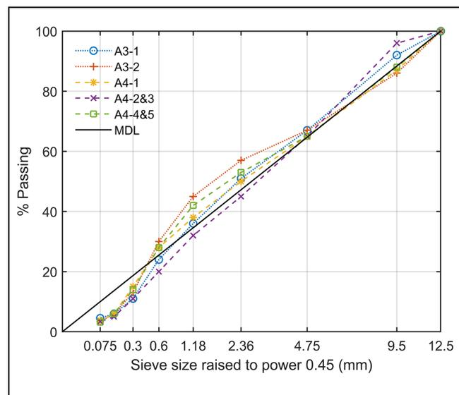
**Figure 1.** Gradation curves of mixtures with nominal maximum aggregate size (NMAS) = 9.5 mm.
